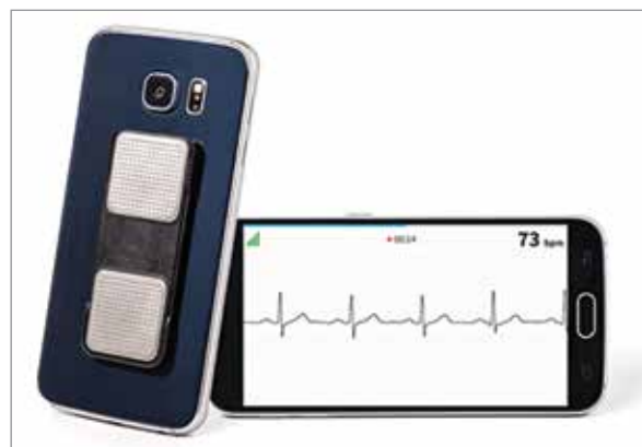
Figure 5. Smart phone attachments and apps are available that can record a single lead ECG to detect arrhythmia. In this example, the mobile ECG device with metal electrodes is attached to the back of a smart phone. The phone is held with the fingertips resting on the metal electrodes to record an ECG.
